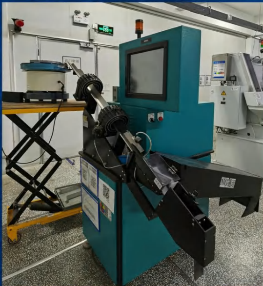
In House Eddy Current Machine is Used to Detect Loose Welding and Cracks on Every Bi-Metal Screws
