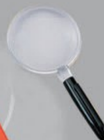
P-20A W/Pen clip Lens dia. 45mm Magnification: 3x Lens material: Acrylic Handle: PP
