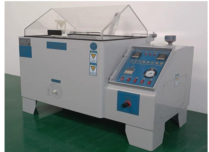
Salt Spray test
